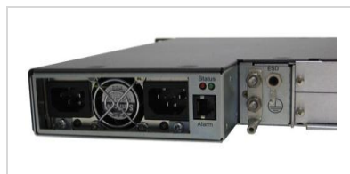
Rear Power Input and Alarming View
